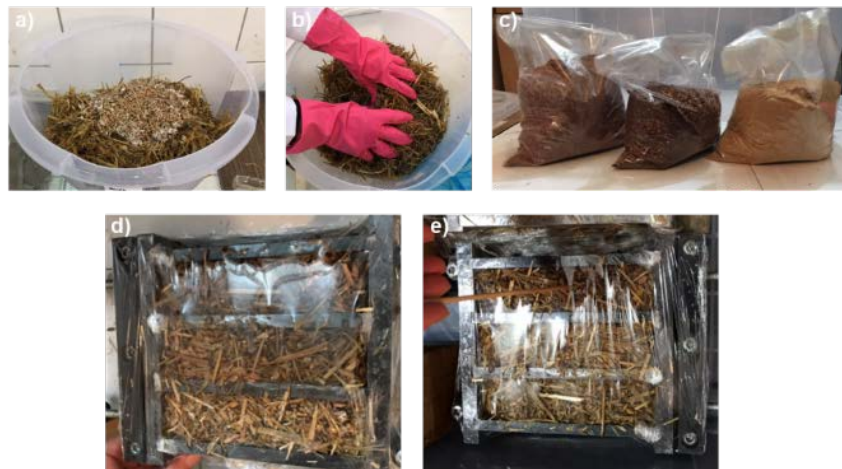
Figure 20 a) Preparing the Mixture According to The Proportions b) Mixing The Mixture c) Samples Kept In The Bag For 7 Days d) Molded Samples And The Prepared Sterile Mold e) Drilling Holes In The Samples After Molding
