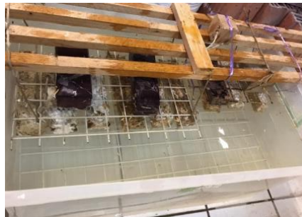
Figure 22 Mechanism Formed for Water Absorption Measurement
