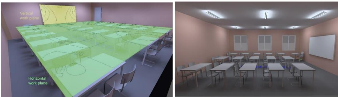
Figure 2 Work planes for calculation
