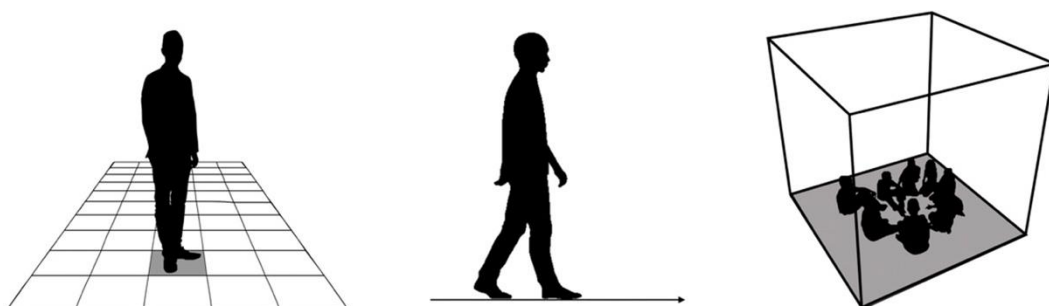
Figure 1 Representations of (left to right) a point, line, and convex space in space syntax (Source: Tannous et al., 2021).
