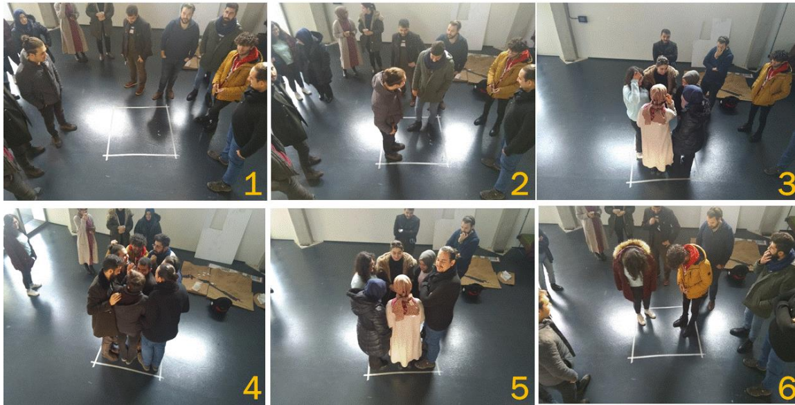
Figure 5 Personal space experiments where a 1x1 square is marked at the floor (1). Afterward, they start to test different loads such as the basic TS 12127 and TS 12186 load (2), crushing loads (3&4) followed by different case studies (5&6).
