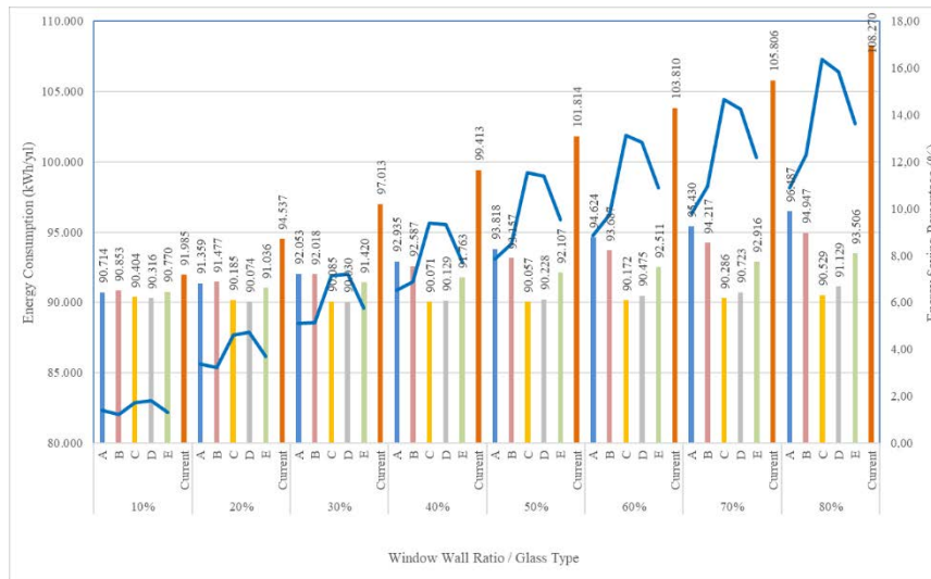
Figure 9 Energy saving rates, calculated energy consumptions and reference energy consumptions for Northeast
