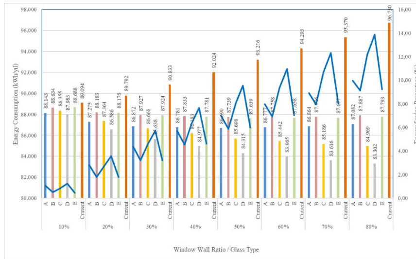
Figure 12 Energy saving rates, calculated energy consumptions and reference energy consumptions for Southwest
