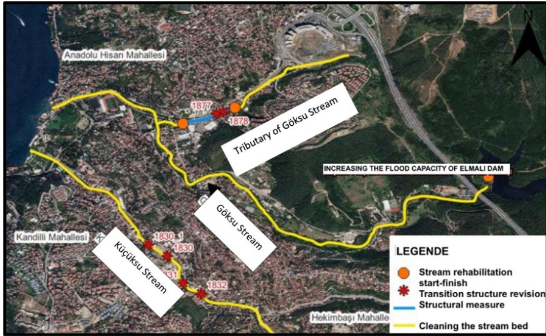
Figure 27 Decisions for Göksu Stream and Elmalı Dam in the Marmara Flood Management Plan (2024)
